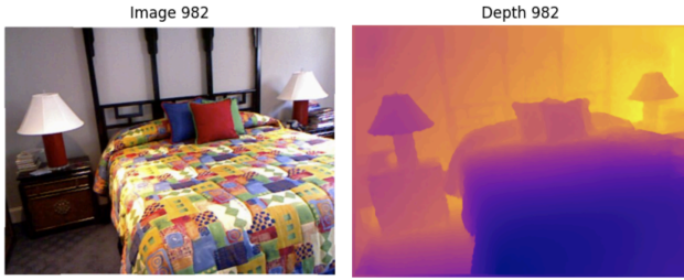
Example of a RGB photo and depth map from the NYU Depth V2 dataset
